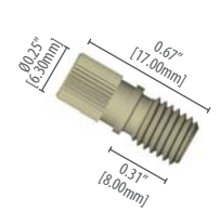
002219 Compact PEEK™ nut for 1/8" OD tubing, 1/4•28
