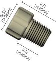
002357 PEEK™ coupling for 1/4•28 F to 1/8" BSPT M threads
