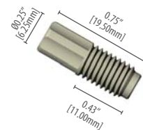
002224 Compact PEEK™ nut for 1/8" OD tubing, 1/4"28
