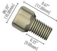
002244 PEEK™ nut for 1/8" OD tubing 1/4•28, natural
