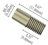
002245 Compact PEEK™ nut for 1/8" OD tubing, 1/4•28
