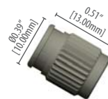
002333 PEEK™ in-line connector for 1/4•28 F threads, 1/16" OD tube
