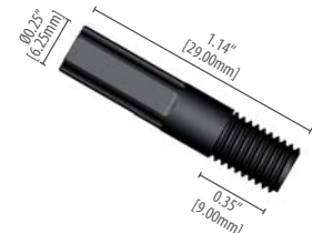
008NF32-YL5B Long nut for 1/8" OD tubing, 1/4•28, black
