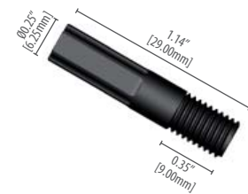
008NF32-YL5B Long nut for 1/8" OD tubing, 1/4•28, black
