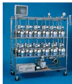
Restek's canister cleaning system with humidification chamber.
