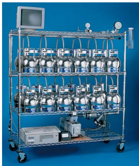
Figure 8 User-designed system for cleaning 24 six-liter canisters.
