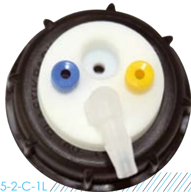
Ref. : SW55-2-C-1L 2 entries 1/8" and 1 barbed to port fitting 90° 8mm and charcoal emplacement
