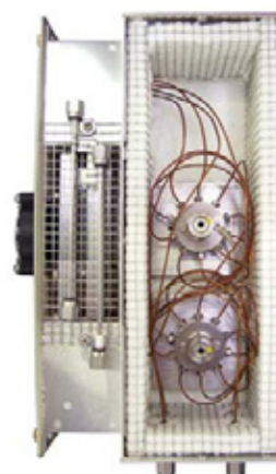
Dual TO-14 Concentrator (four traps, two valves)
