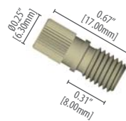
002119 Compact PEEK™ nut for 1/16" OD tubing, 1/4•28
