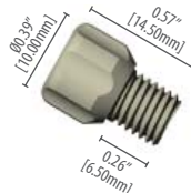
002222S PEEK™ nut for 1/8" OD tubing, 1/4•28
